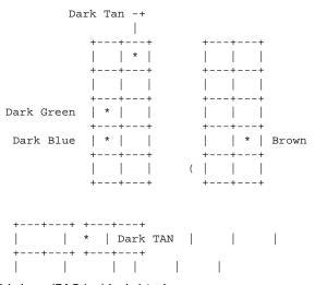
The Dark TAN wire connects to a pressure sensitive switch on the brake master cylinder. This wire gets connected to the Dark TAN wire of the Cluster connector and is used to turn on the BRAKE light if the line pressure in the master cylinder drops below a safe level, (indicating loss of fluid, internal seal failure, or open brake line.)
